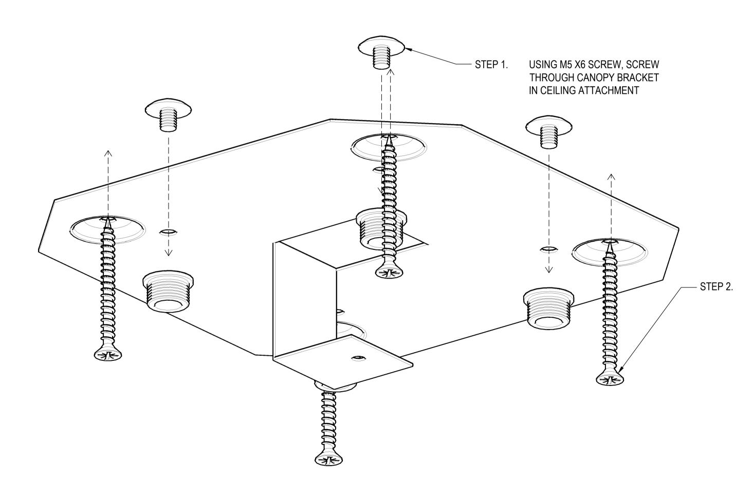
USING GENERIC TIMBER SCREWS, SCREW INTO CEILING, NOTE: USE CORRECT CEILING SCREWS FOR TYPE OF CEILING. FITTING SHOULD BE SCREWED INTO TIMBERS IN THE CEILING (SCREWS NOT SUPPLIED)
